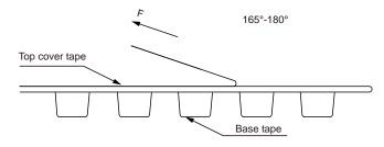
The peel force of top cover tape shall be between 0.2 to 0.58 N  $\,$
