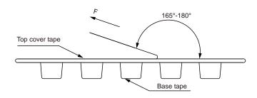
The peel force of top cover tape shall be between 0.14 to 0.58 N
